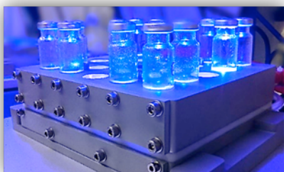
Fig. 6 - High-throughput screening photoreactors (HTSP)
